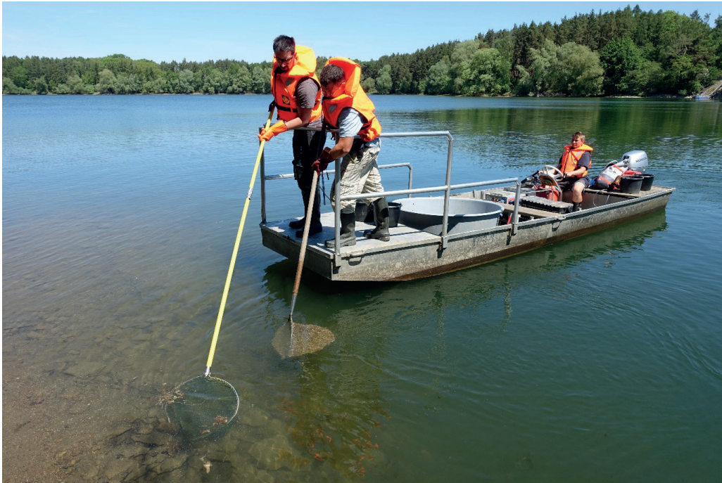
Figure 4.2. Point abundance fishing for fry from a boat. The positive anode (circular shape) at the end of the fibreglass rod is placed in the water in front of the boat and at the same time, the electric field is activated by foot switch. All stunned fish are then collected by an operator with a landing net (photo: Petr Blabolil).
