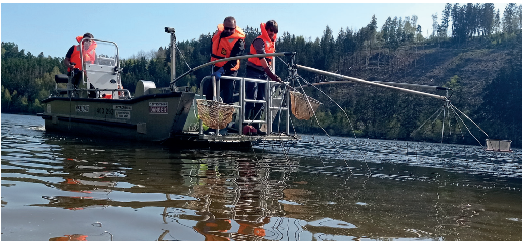
Figure 4.1. Continuous boat electrofishing using two anodes in front of the boat, where the metal boat construction serves as the cathode (photo: Ivana Vejříková).
